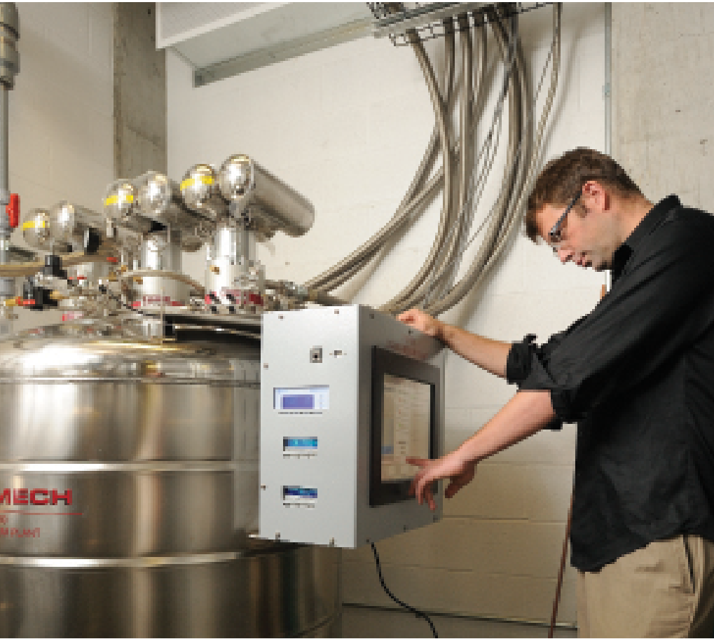
Assistant Professor N. Peter Armitage makes adjustments to the new helium reliquefier system.
